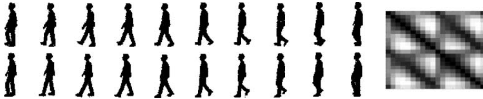
Gait Recognition, Motion Analysis for. Figure 1 Twenty sample frames from a walking cycle from a side view. Each row represents half a cycle. Notice the similarity between the two half cycles. The right part shows the similarity plot: each row and column of the plot corresponds to one sample. Darker means closer distance and brighter means larger distances. The two dark lines parallel to the diagonal show the similarity between the two half cycles.
